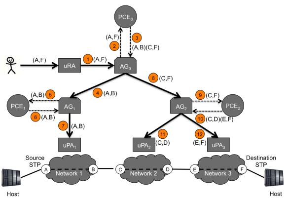
Figure 2. Example of a tree-based source routing workflow
