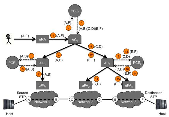
Figure 3. Example of a tree-based source routing workflow
