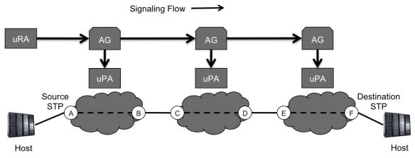
Figure 4. Chain-based signaling flow
