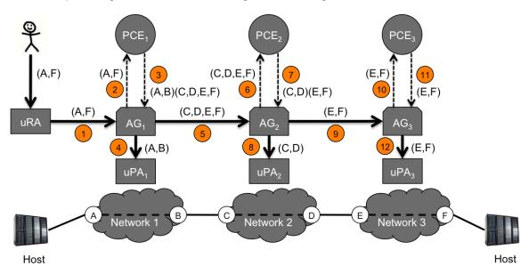
Figure 6. Example of a chain signaling workflow using source routing
