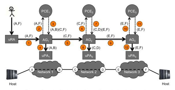
Figure 5. Example of a chain signaling workflow using hop-by-hop routing
